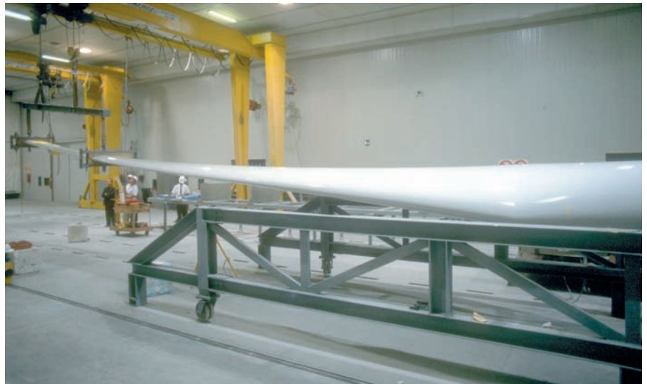
Testing for maximum deflection at the tip
