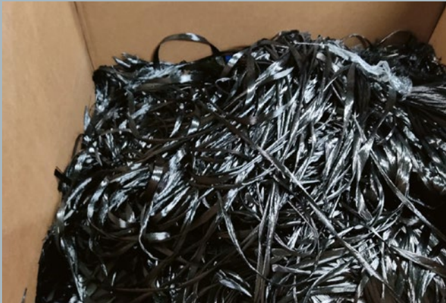
A local company takes bobbin ends of unused carbon fiber and uses our waste to produce a thin carbon textile (Spain)
