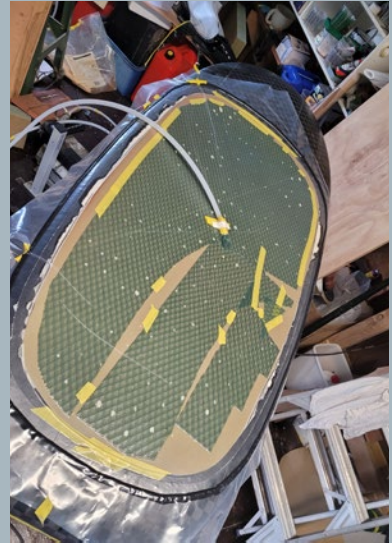
Too thin for most applications, the foam core skims leftover after processing are highly suitable for wingfoil board production (New Zealand)
