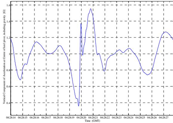
Figure 9 : Vertical acceleration time history for a typical slam on Wild Oats
