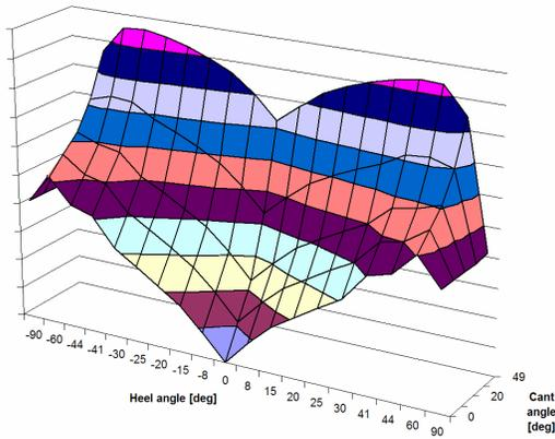
Figure 2 : Calculated forward keel pin lateral loads on a 60 foot canting keel boat using SP sailing load cases
