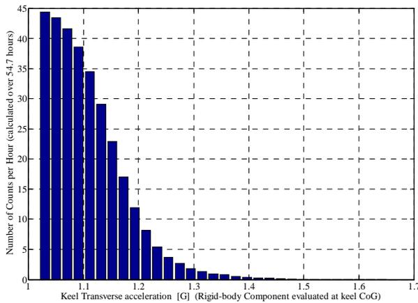
Figure 6 : Histogram of rigid body keel bulb accelerations on Wild Oats. The number of counts corresponds to the average number of instances per hour when the keel acceleration exceeds the given value.
