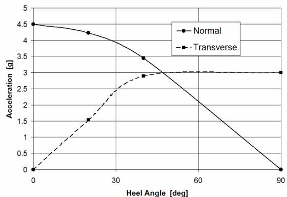
Figure 1 : Typical SP design acceleration envelope for a 60 foot canting keel boat. The ‘Normal’ component always acts parallel to the yacht vertical axis, and the ‘Transverse’ parallel to the boat transverse axis.
