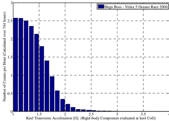
Figure 5 : Histogram of rigid body keel accelerations on Hugo Boss. The number of counts corresponds to the average number of instances per hour when the keel acceleration exceeds the given value.
