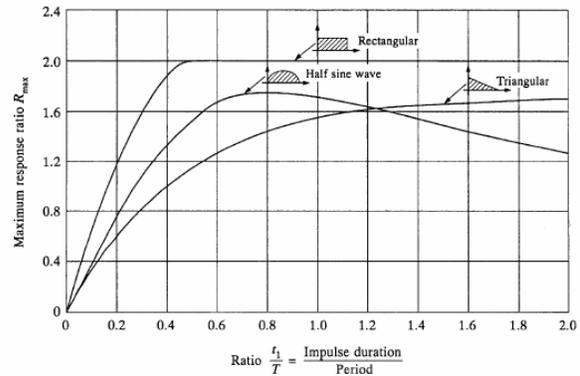
Figure 11 : Dynamic response spectra of a single-degree-of-freedom system to impulse load [8]
