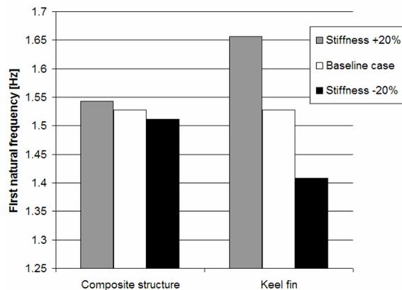
Figure 14 : Effect of composite structure and fin stiffness on keel structure natural frequency.
