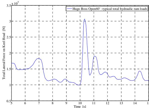
Figure 8 : Keel ram load time history for a typical slam on Hugo Boss
