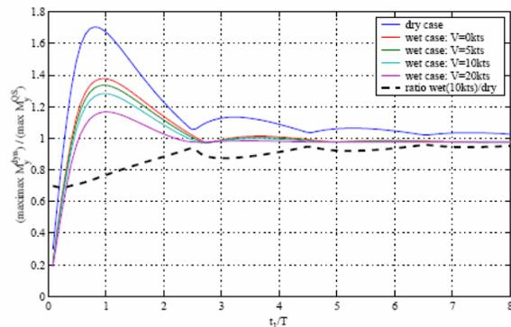
Figure 12 : Open 60 theoretical shock spectra: bending moment at keel root for half sine shaped transverse acceleration impulse [7]
