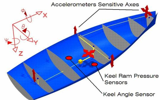
Figure 3 : Typical layout of data acquisition sensors
