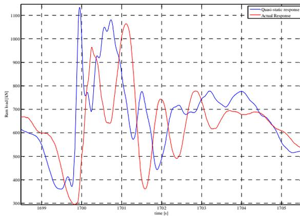
Figure 10 : Keel ram load time history for a typical slam on Wild Oats. The measured response (red line) is compared here with the load calculated using quasi-static assumptions (blue line).
