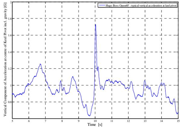
Figure 7 : Vertical acceleration time history for a typical slam on Hugo Boss
