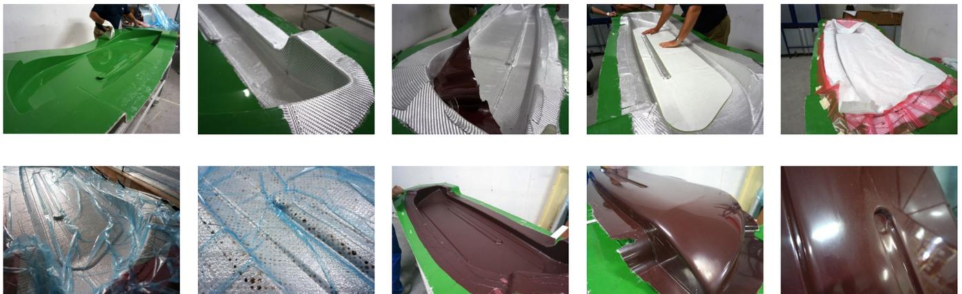
Figures 1 – 10: The 'one-shot' lay-up and curing process from start to finish
