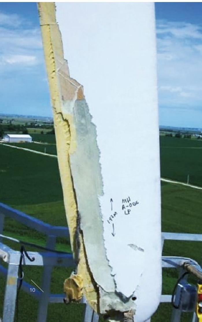
erosion, critical bonding areas to start separating or even more compromising damage to the composite structure. Any of these critical components will likely render the turbine inoperable for some time and the current repair solutions are critically impacted by temperature and humidity, reducing the repair teams' access to the turbines throughout the year.
