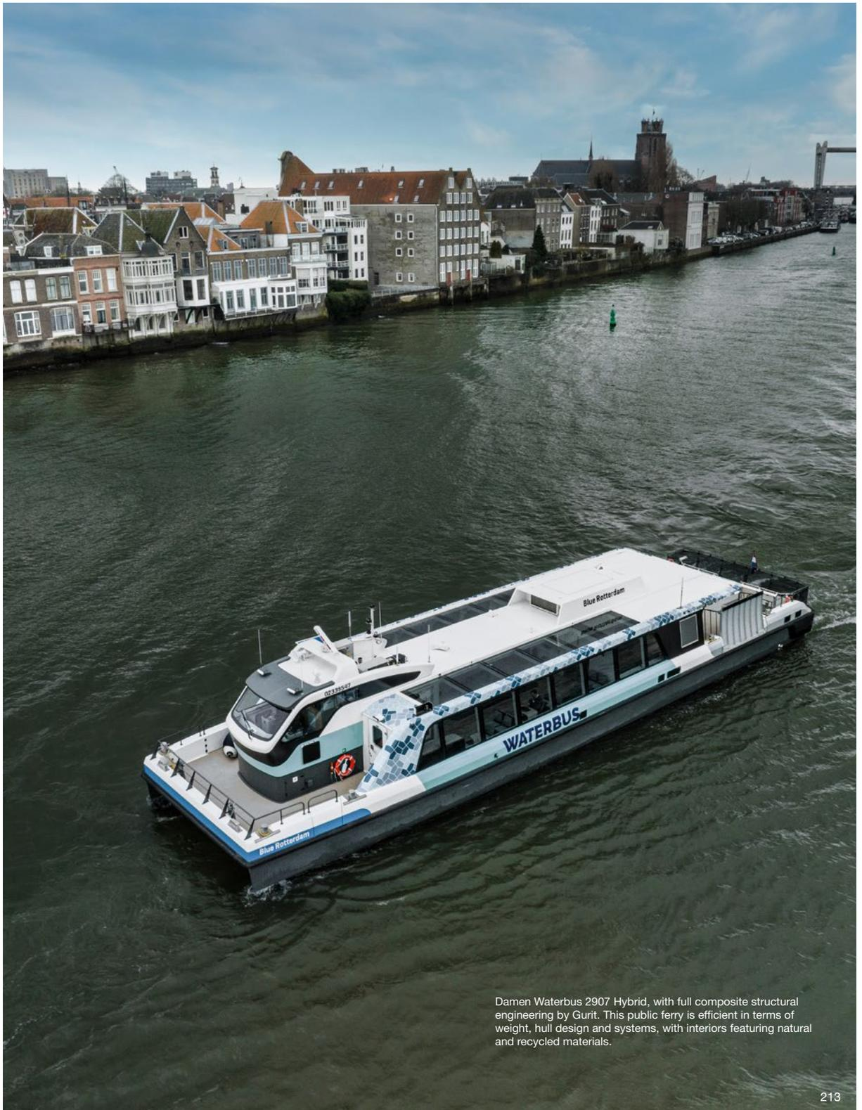
Damen Waterbus 2907 Hybrid, with full composite structural engineering by Gurit. This public ferry is efficient in terms of weight, hull design and systems, with interiors featuring natural and recycled materials.
