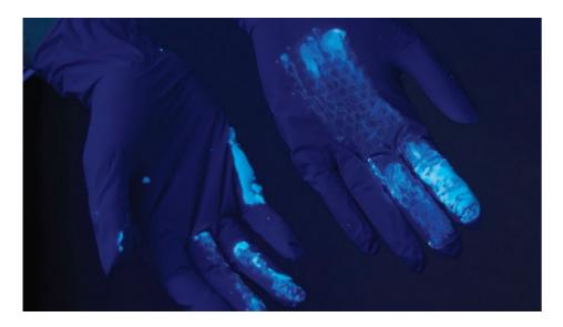
Droplets of resin less than 1mm can be detected by this new approach and high contrast optimised image analysis may increase this further. This allows users to detect contamination from epoxy resin systems both on users' skin and equipment, door handles, and the like that would previously be undetectable with the naked eye.
