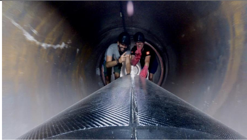
EPFLoop team with the 2018 carbon fibre pod for minimal weight
