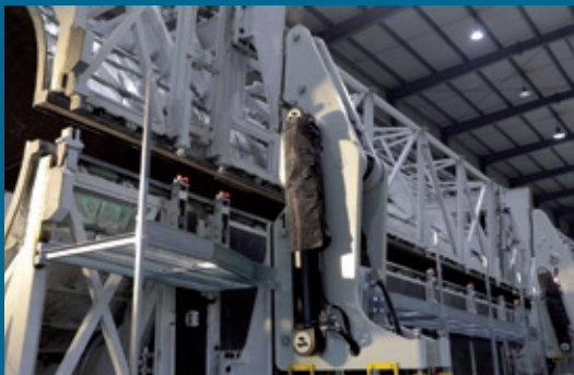
Tooling production in Taicang, China: layout of heating wires for a wind blade mould.
