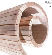
Balsa's native range is from Central to South America. However, Ecuador's location and unique climate create the perfect conditions to give Ecuadorian balsa the best physical and mechanical properties for the composite industry.
