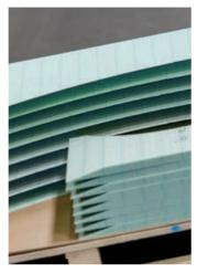
Through smart engineering, we have developed standard chamfers into our kitting designs. Not only does this benefit the customer and their build process, but also reduces waste and the amount of PET needed for the kit, plus enables us to package the kits more efficiently. This innovative improvement allows to transport a larger number of kits in the same space.
