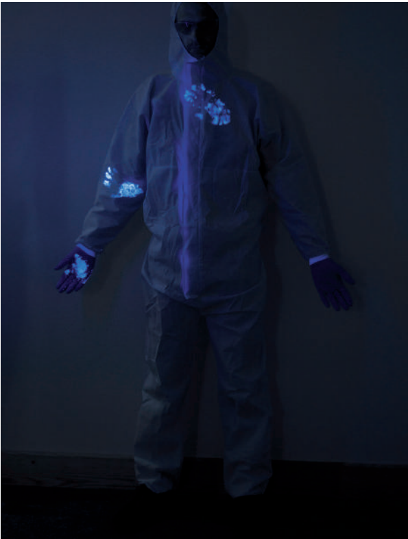
Gurit Light Reflective Technology (LRT) is an optional additive that has been introduced in order to reduce workers' exposure to hazardous chemicals by means of a simple UV-lamp. The additive to the resin matrix can be applied to any laminating and adhesive system without changing their mixing and handling properties or cured resin performance.
