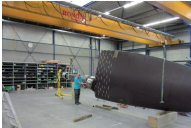
Dutch shipyard Royal Huisman: largest superyacht rudder ever built.
