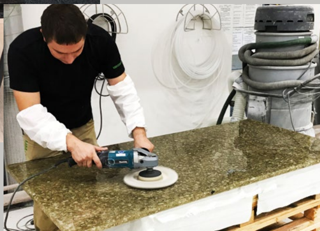
Polishing a table plate produced from recycled composites
