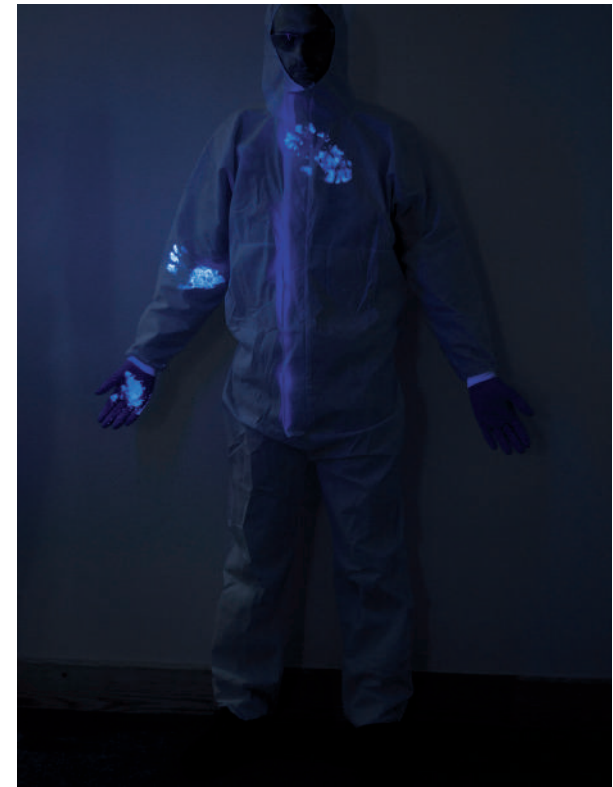
Gurit Light Reflective Technology (LRT) is an optional additive that has been introduced in order to reduce workers' exposure to hazardous chemicals by means of a simple UV-lamp. The additive to the resin matrix can be applied to any laminating and adhesive system without changing their mixing and handling properties or cured resin performance.
