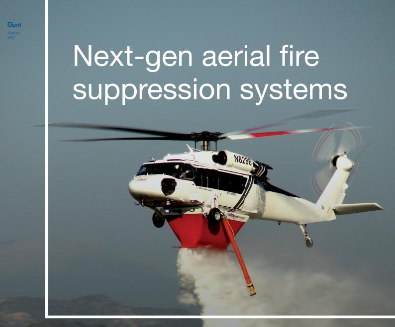
Helitak is a firefighting specialist, designing and manufacturing rotary aerial firefighting equipment. With well over a decade of research and development, Helitak has developed an efficient, compact, reliable and cost-effective fire tank, constructed with advanced composite materials from Gurit.
