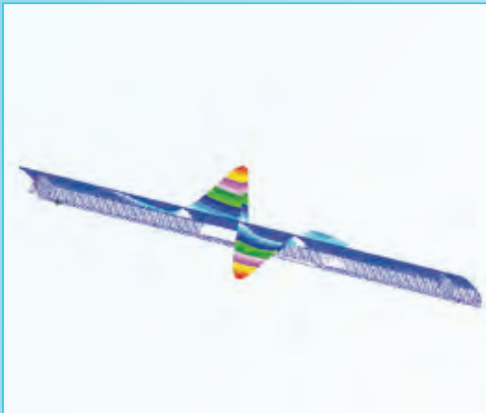
Finite Element Analysis was used by Gurit in its research into the buckling stability of a furling boom.
