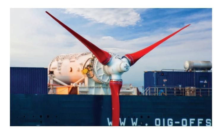
With a rated capacity of 1MW and a diameter of over 20m the ANDRITZ HYDRO Hammerfest HS1000 is the largest single tidal turbine rotor to be installed to date. The 9m tidal blades were engineered and manufactured using Gurit materials by a team at Gurit UK.
