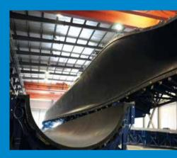
As wind turbines become ever larger and more powerful, so too do the moulds used to manufacture the turbine blades. The recent expansion of its production halls has made Gurit Tooling capable of manufacturing moulds of to 100 meters in length. In 2014, the longest mould produced by Gurit almost reached this scale. It was a mould to manufacture blades that were 88 meters long. A truly gigantic tool!
