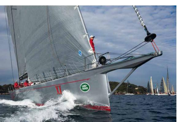
last Twin Foil CBTF technology, allowing it to carry a massive sail area without compromising on stability. Gurit's Engineering team provided the detailed design and analysis for the vessel's composite structure and met the structural requirements of this original design by specifying its SE 84 carbon prepreg combined with Nomex cores throughout, to achieve an all up displacement (weight) of 30.6 tons.
