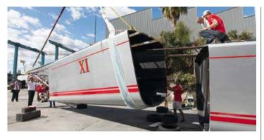
sold to a new owner from California and has recently undergone a major refit for a new life of very different racing on the US West Coast. Now named Rio 100, it was chosen because it does not have a canting keel. Instead it relies on a fully manual winch system. The focus of the changes to the yacht have been to turn it into a yacht optimized for VMG (Velocity Made Good) running in light to moderate conditions, as expected in the Transpacific Yacht Race and US West Coast races.
