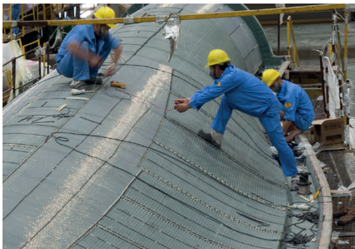
Installation of a mould heating system at the Gurit Tooling premises.
