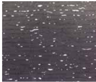
With standard prepreg voids form between plies. Void content 3.25%
