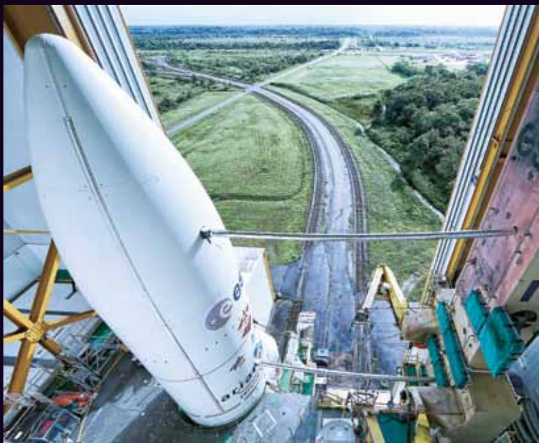
The ogive shaped payload fairings which form the top end of the rockets and protect the cargo during the flight through the atmosphere are made with Gurit materials.
