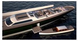
Early rendering of main hull door<sup>1</sup> 1 renderings courtesy of Design Unlimited With Naval Architecture by Judel/Vrolijk this vessel stands out not only by the fact that, once launched, it will be the largest carbon fibre sloop in the world, but also due to the presence of a rather unique design feature; a pair of large balcony doors cut into the topsides; one forward, acting as a balcony to the master cabin, and one amidships serving as a tender dock and main sea entrance.
