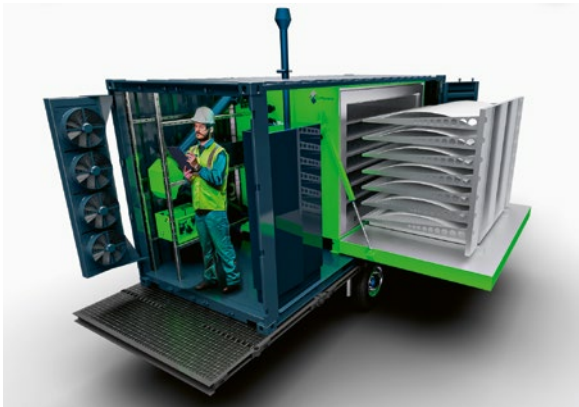
Render of Composite Recycling's proposed container-sized pyrolysis centres
