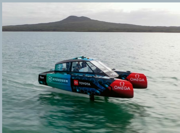
Chase Zero, a pioneering hydrogen vessel made with Gurit composite materials and composite structural engineering support
