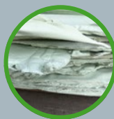
PET WASTE FROM EXTRUDER START-UP/ SHUT-DOWN
