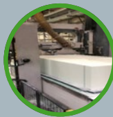
PET WASTE DUST COLLECTED BY OVERHEAD PIPING
