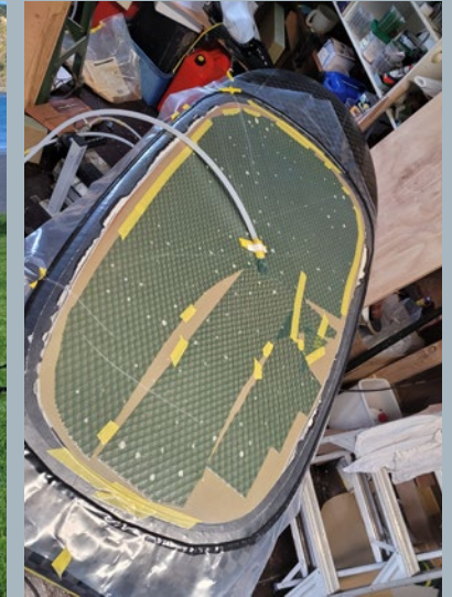
Too thin for most applications, the foam core skims leftover after processing are highly suitable for wingfoil board production (New Zealand)
