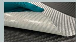
ST90 single sided SPRINT™ is a moulding material that consists of a layer of dry reinforcement applied to a pre-catalysed resin film. Standard T1 variants suit use in temperatures below 25°C (77°F), the T0 variant available on request is more suitable in temperatures of 25°C (77°F) and above. Cured properties are the same for both tack variants.
