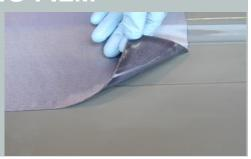
SF 75-90 surfacing film is a filled epoxy film with glass carrier. It forms an easy to sand surface ideal for paint application.
