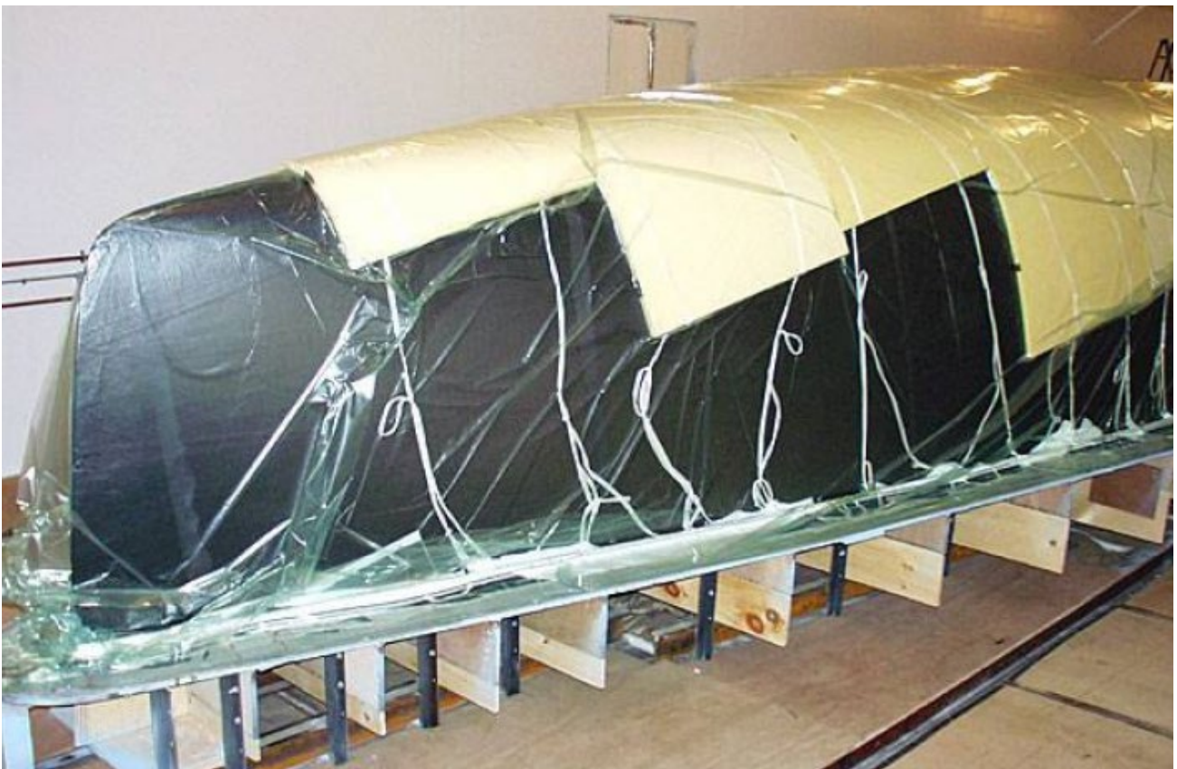
Figure 1 - Thermo-forming core over a male molded yacht hull
