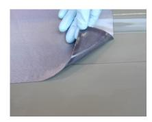
The material can be placed into the mould in any size/shape however it is important to keep overlaps to an absolute minimum, butt joins are ideal.
