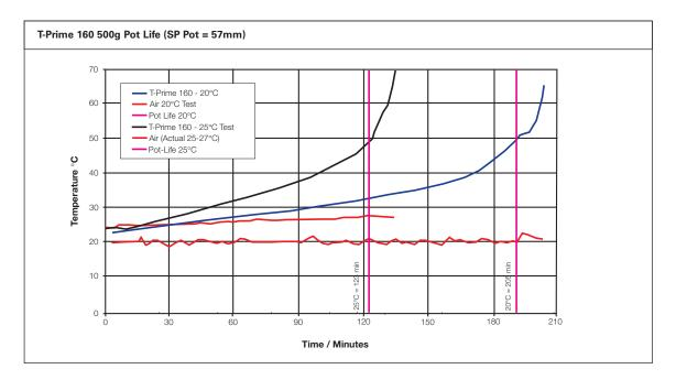
Large volumes of T-Prime 160 left in a pot can exotherm strongly and remaining mixed resin will need to be dispensed into a shallower vessel towards the end of the pot-life. Ideally the remaining resin should be less than 30mm deep or the pot placed into water to cool. Both the 20°C and the 25°C sample in this test (57mm deep) produced smoke at the end of the pot-life from the large exotherm temperature.
