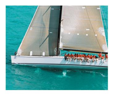
Gurit met the structural requirements of this design by specifying SE 84 carbon prepregs combined with Nomex cores throughout to achieve an all up structural weight of less than 2 tonnes and an all up sailing weight of just 11 tonnes. By combining experience in Open 60 class racing yachts and several large racers and racer cruisers, Gurit was able to design a fully composite canting keel structure that houses the entire keel mechanism without unduly obstructing the interior.
