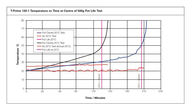
Large volumes of T-Prime 130-1 left in bulk > 50mm deep can exotherm strongly and the excess will need to be dispensed into a shallower vessel. Ideally this should be less than 30mm deep or the pot placed into water to cool.
