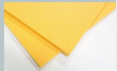
Gurit<sup>®</sup> Corecell<sup>™</sup> M is the high-performance foam, featuring extremely high resistance to impact, slamming and fatigue, suitable for all marine applications across all sectors. Combining high static properties, unmatched toughness, and compatibility with infusion, prepreg, SPRINT<sup>™</sup> and wet lamination processes.
