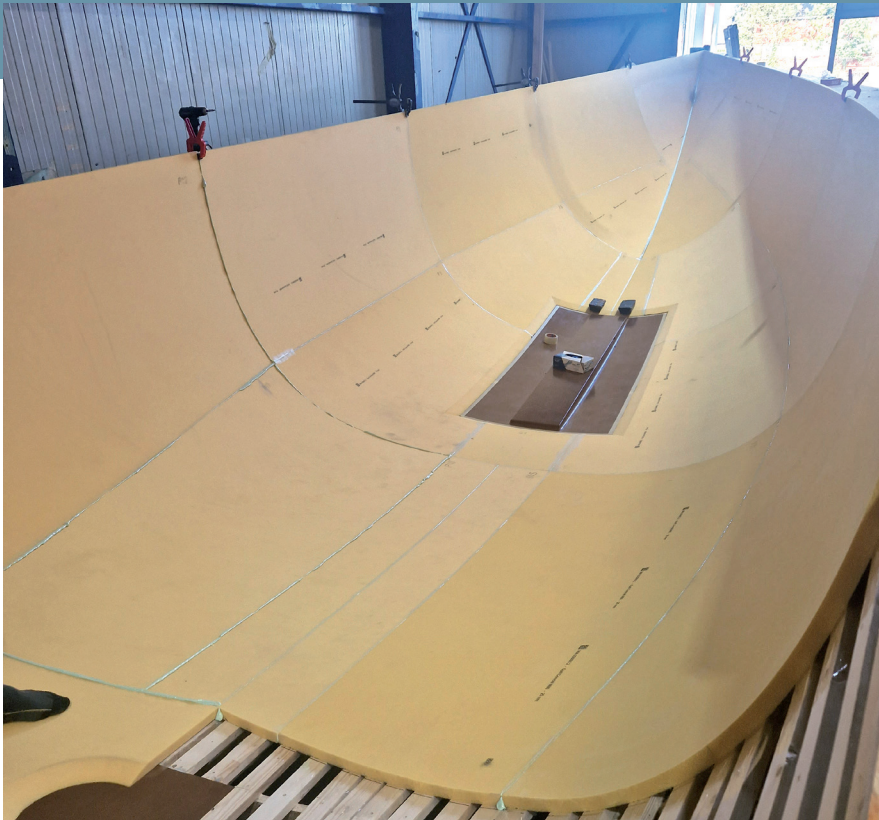
3D Core Kit bonding and assembly of wooden jig
