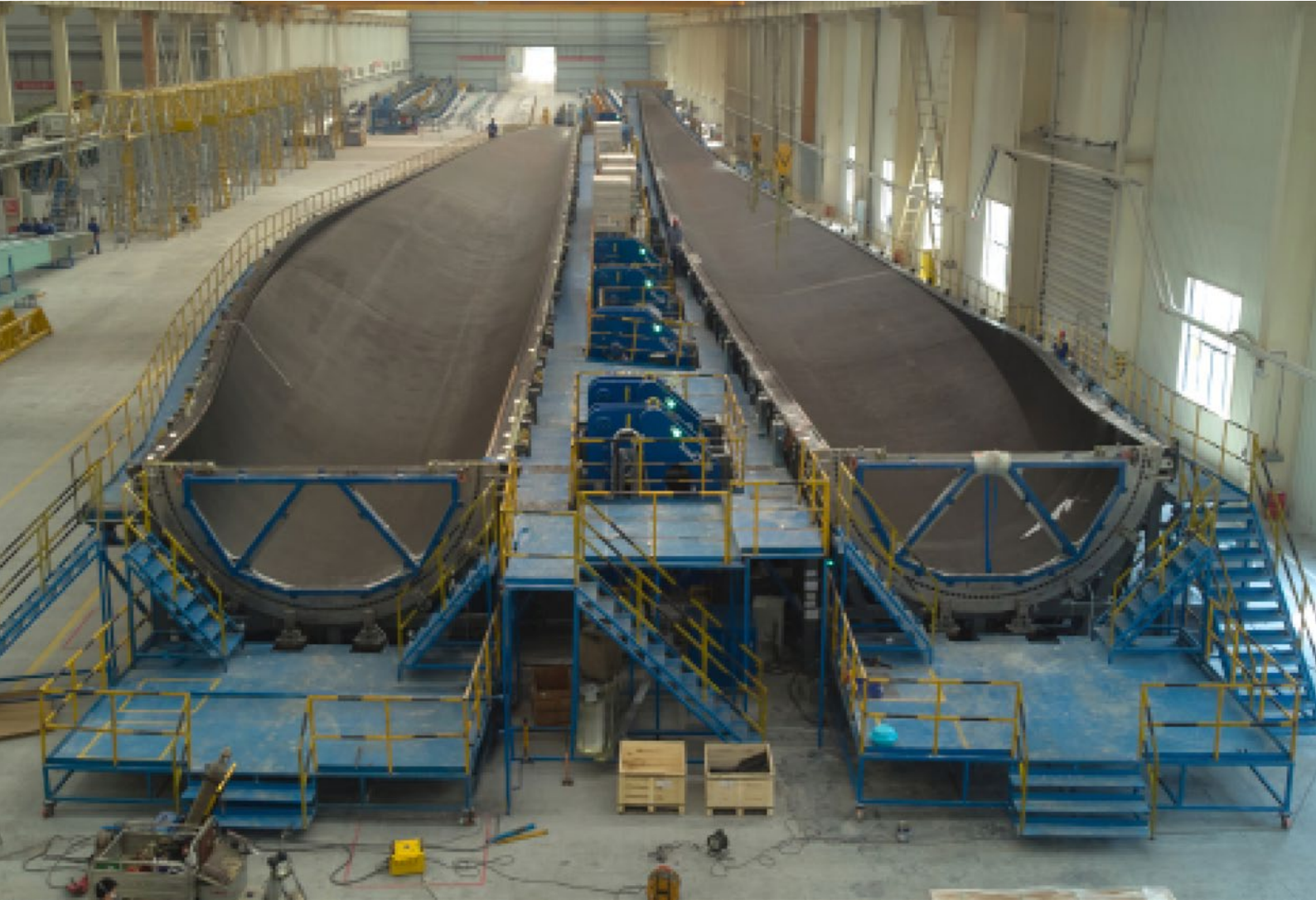
One of the world's longest wind turbine blade moulds in build at Gurit Taicang
